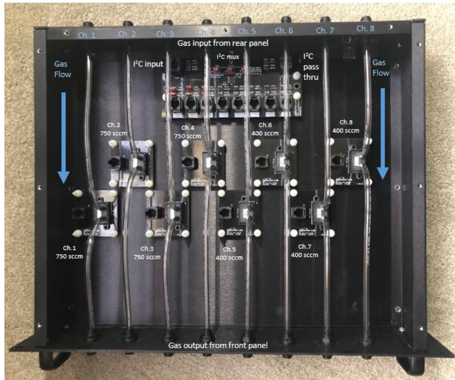
View of the DSG designed gas flow sensor chassis
